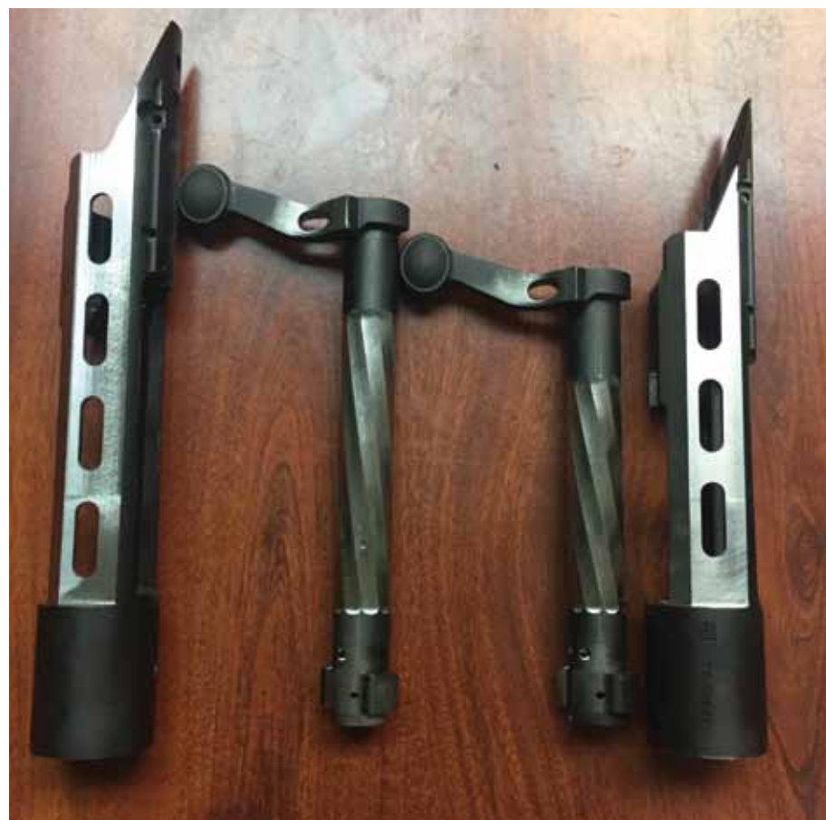
It's easy to see the difference between a long action and short action when the rifle is taken apart.
