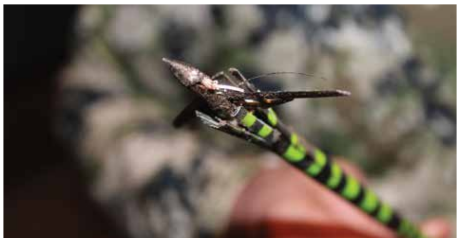
When this mechanical broadhead struck the thick shield of a mature wild boar it was driven back into the shaft and never penetrated into the vital area. This incident convinced the author to use a fixed broadhead on the Airbow.
