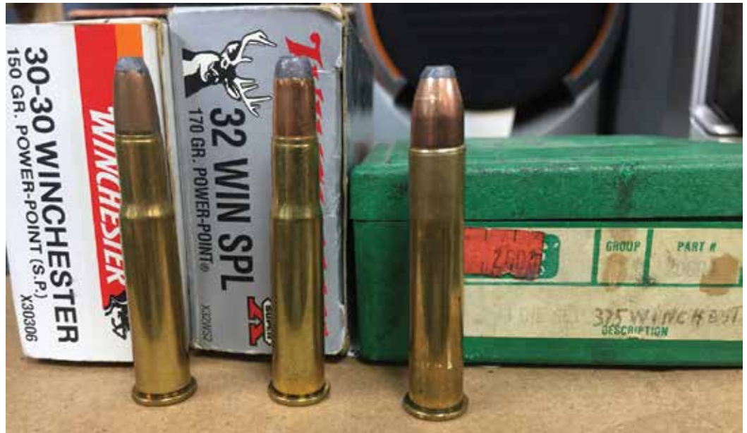
Finished loaded rounds include, (left to right) 30-30, 32 Win. SPL and 375 Win.
