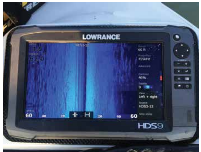
Side scan imaging allows views to the right and left of the craft.
