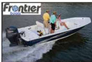
21'5" Mod V Hull 8'3" beam. Design Carolina flare bow shape, self-bailing deck, hand laid hull & cap. Locking rod storage, premium upholstery
