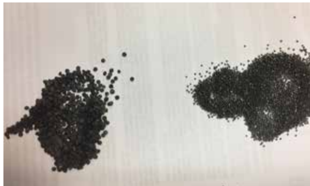
The ball powder on the right is more abrasive than the flake powder.
