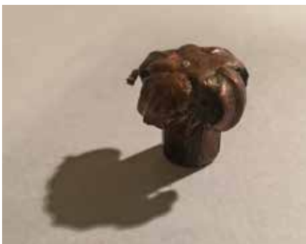
A perfectly expanded Barnes 30 cal bullet that was removed from a bezoar ibex shot at 450 yards.
